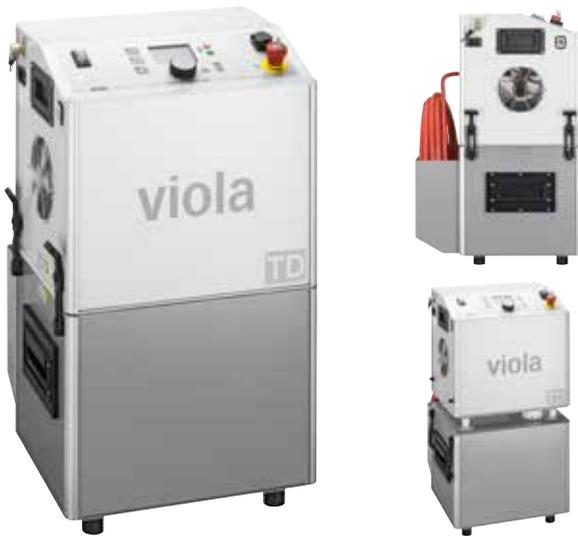
The portable, high performance viola high-voltage testing and diagnostics device is available in two different configurations. The standard variant is used for cable and cable sheath testing of electrical equipment and medium-voltage cables up to 35 kV. Another function is insulation testing on electrical equipment. The patented VLF-truesinus® technology (0.1 Hz sine voltage) guarantees a high level of measurement accuracy.
