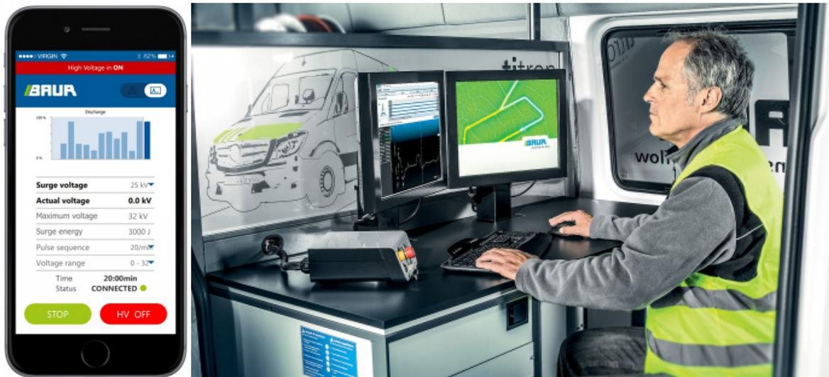
*Remote control via app: The surge voltage generator of the titron cable test van can be started and stopped for the cable fault pin-pointing via the smartphone. This way, the cable route is not loaded with high voltage pulses for longer than necessary.*
