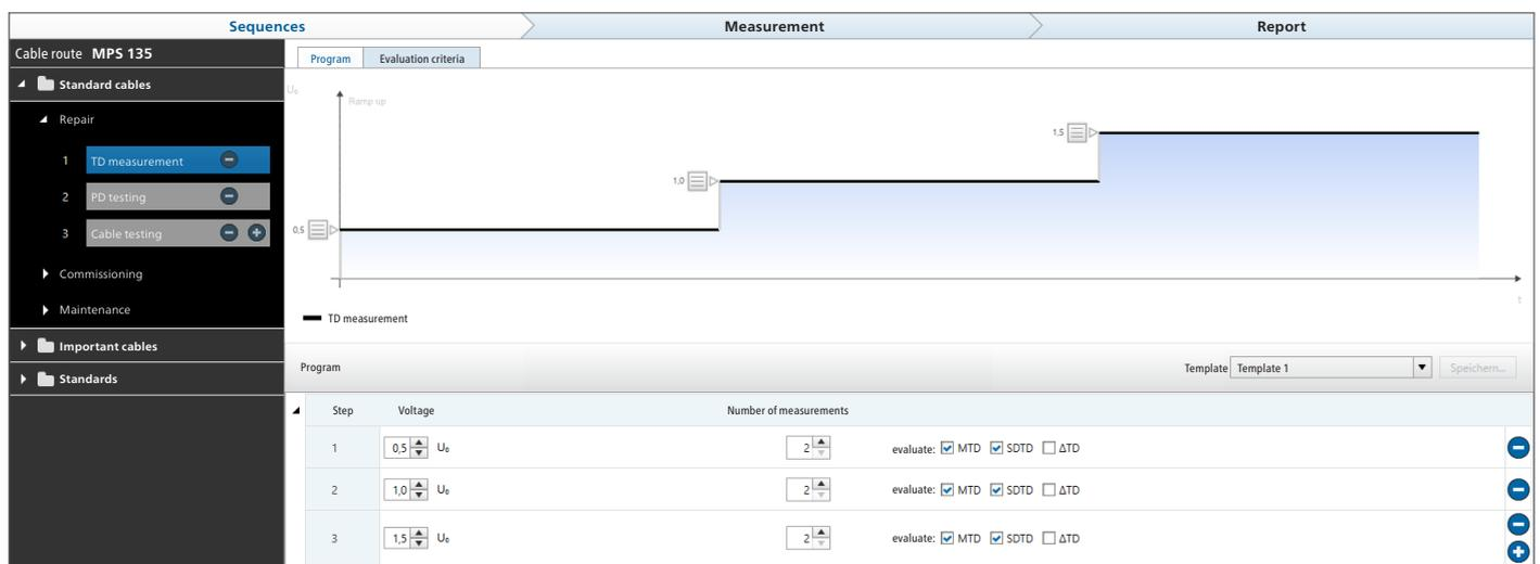
Example: Configuration of a dissipation factor measurement within a sequence
