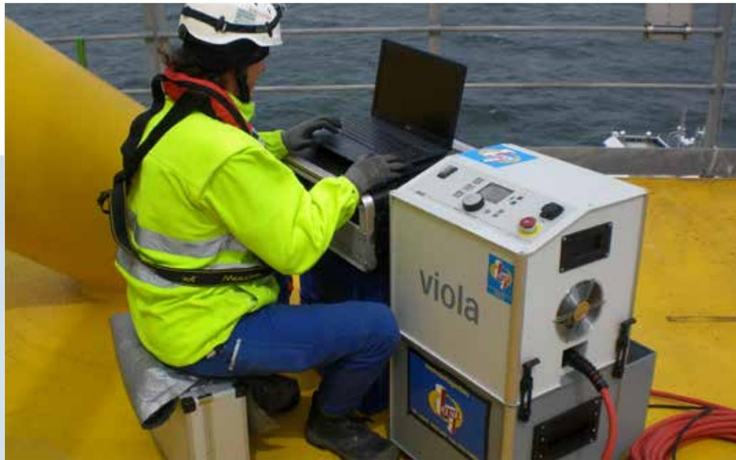
After about 2.5 hours, the job at this wind turbine is done and it's on to the next one. The measurement results are "in the box", according to Wenzel. "The device displays the test status immediately and we can notice any irregularity." In addition to the test results, the log shows the external temperature and humidity, the torque with which the terminations were tightened and finally the calibration dates of the torque wrench and tester.
