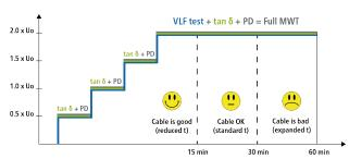
insulation. Moreover, a partial discharge measurement shows and locates the PD faults precisely. The highlight of MWT is the condition-based test duration: Provided it is permitted, the test duration can be shortened, which in turn lowers costs. This way, the cable is only exposed to the increased test voltage for the required duration.
